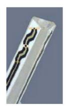
Figure 2.3 Probe Thick-Film Technique
