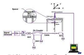
**Figure 7.1 Dipole Validation Test Setup**
