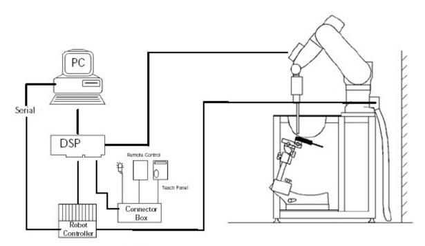
Figure 2.1 SAR Measurement System Setup
