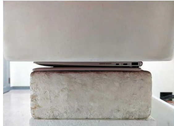
Fig.3 EUT Back side to flat phantom
