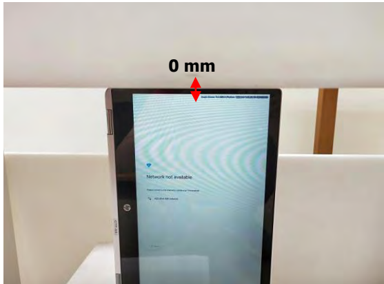
Fig.7 EUT Left side to flat phantom
