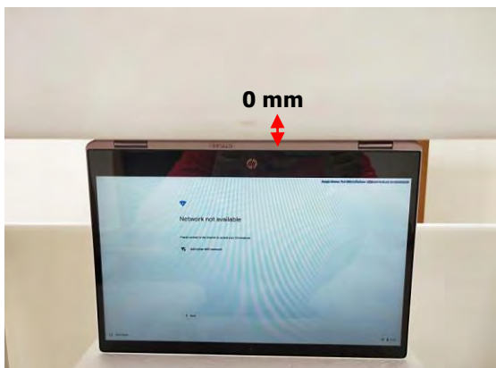
Fig.5 EUT Bottom side to flat phantom
