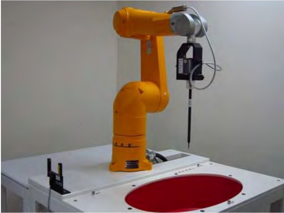
Fig.1 Photograph of the SAR measurement system
