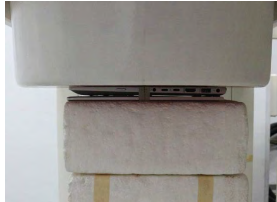
Fig.3 EUT Back side to flat phantom
