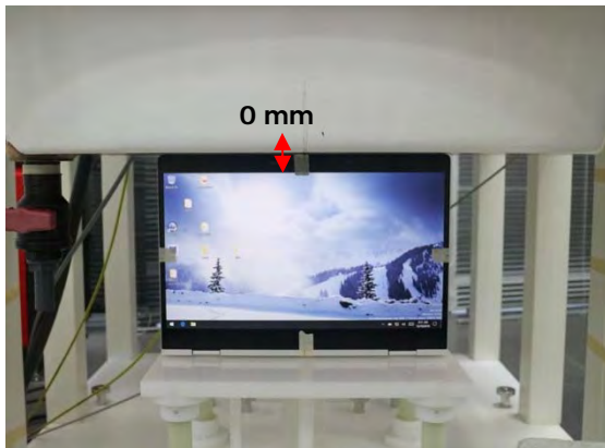
Fig.4 EUT Top side to flat phantom
