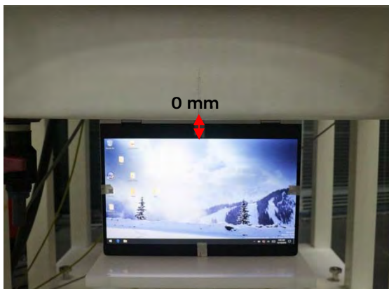
Fig.5 EUT Bottom side to flat phantom
