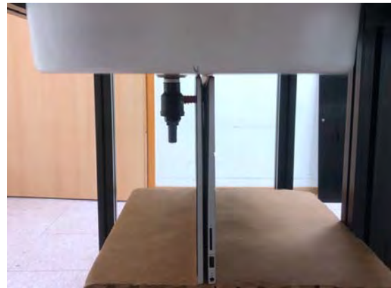
Fig.4 EUT Top side to flat phantom
