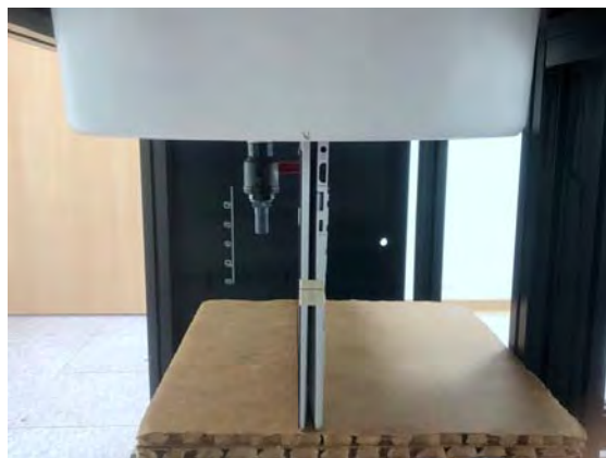
Fig.5 EUT Bottom side to flat phantom
