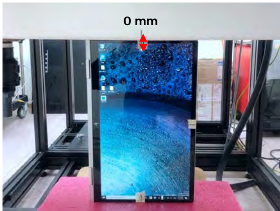
Fig.7 EUT Left side to flat phantom
