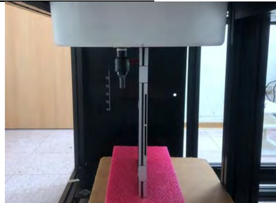
Fig.6 EUT Right side to flat phantom
