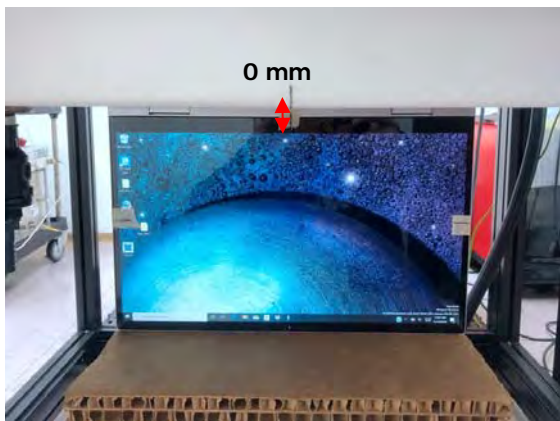
Fig.5 EUT Bottom side to flat phantom
