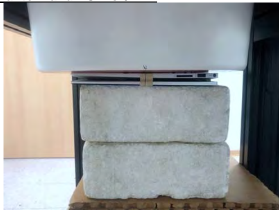
Fig.3 EUT Back side to flat phantom
