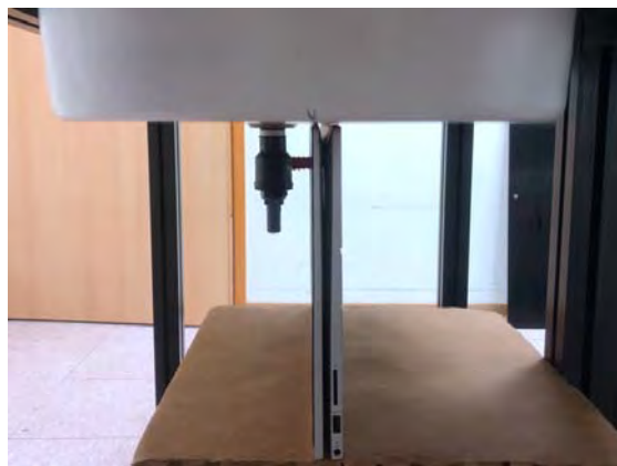
Fig.4 EUT Top side to flat phantom
