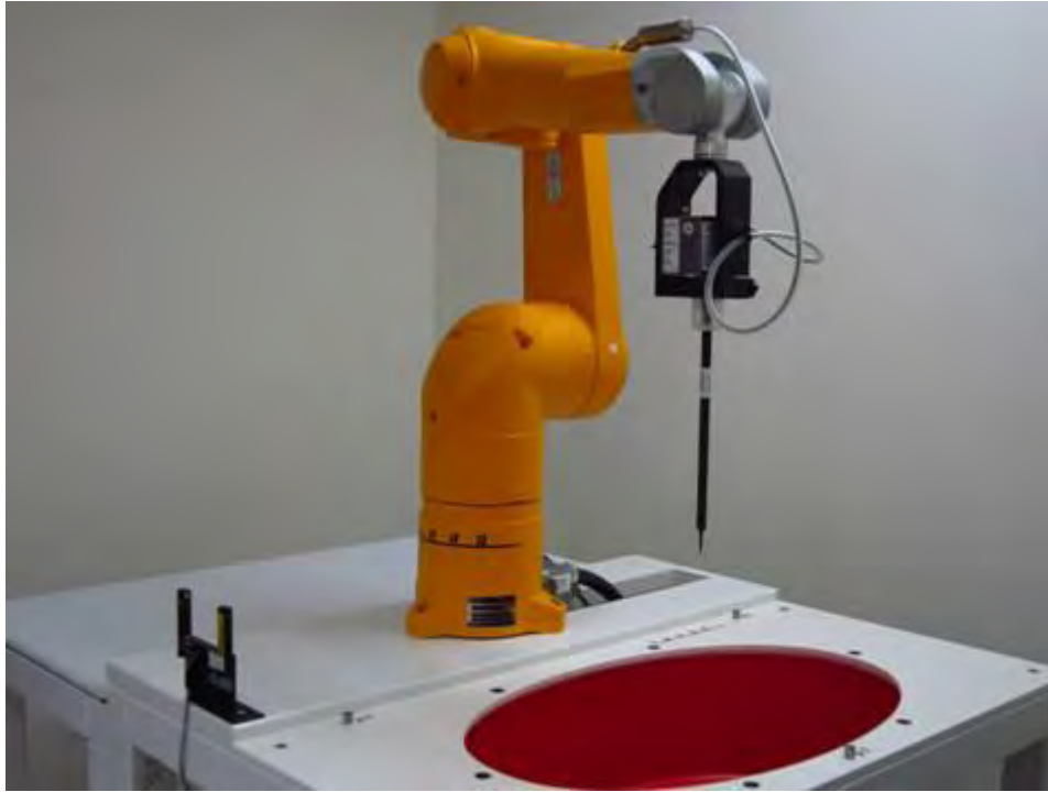
Fig.1 Photograph of the SAR measurement system
