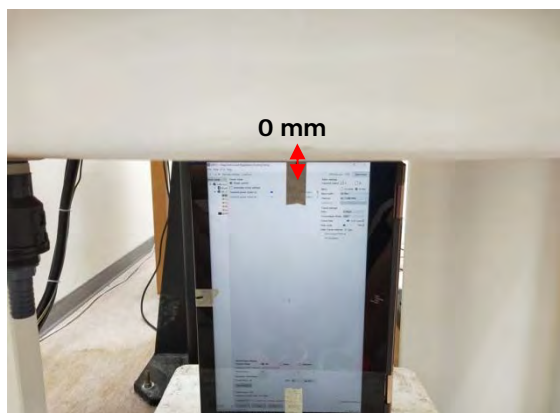
Fig.6 EUT Right side to flat phantom
