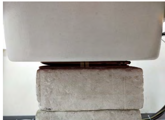
Fig.3 EUT Back side to flat phantom
