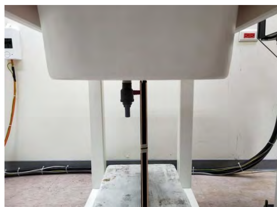
Fig.7 EUT Top side to flat phantom
