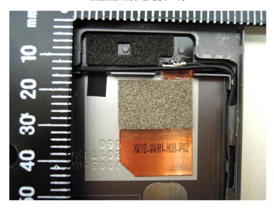
BT / WLAN (Aux) / WLAN (Main) Antenna
