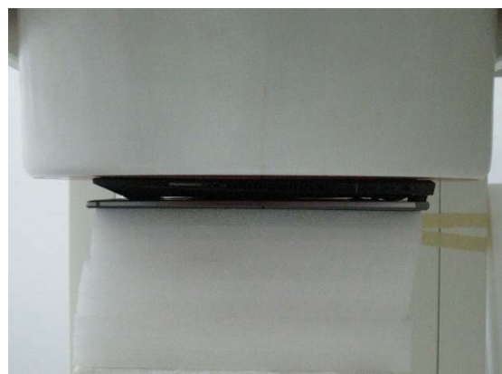
Fig.3 EUT Back side to flat phantom
