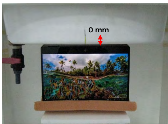
Fig.5 EUT Bottom side to flat phantom
