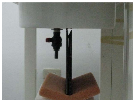
Fig.4 EUT Top side to flat phantom
