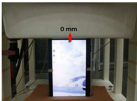
Fig.6 EUT Right side to flat phantom
