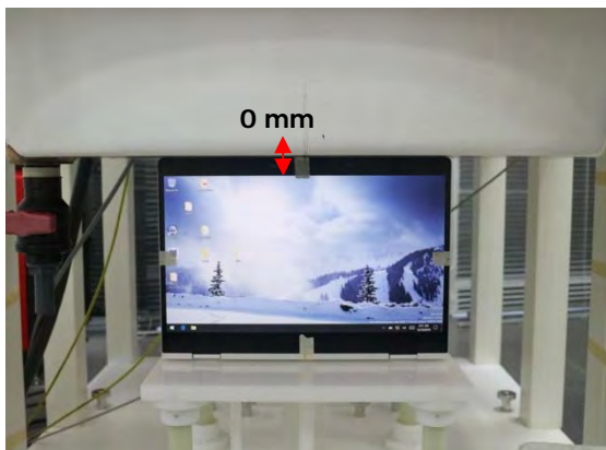
Fig.4 EUT Top side to flat phantom
