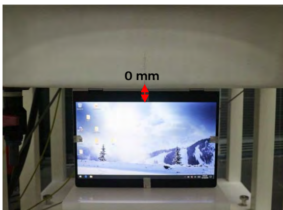
Fig.5 EUT Bottom side to flat phantom
