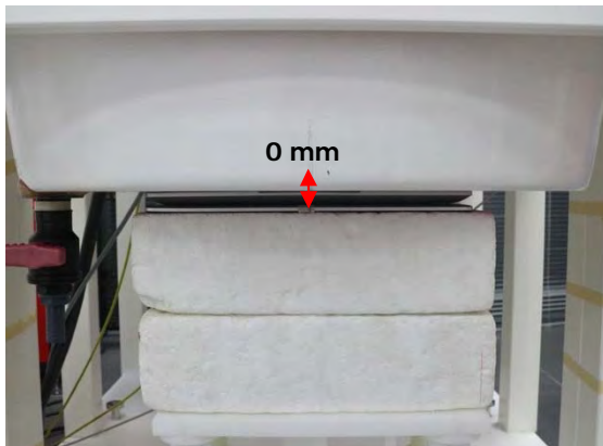
Fig.3 EUT Back side to flat phantom
