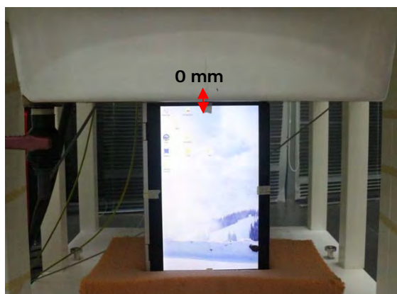
Fig.7 EUT Left side to flat phantom
