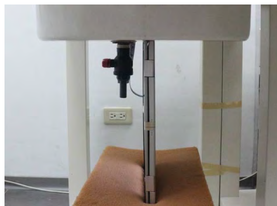
Fig.6 EUT Right side to flat phantom
