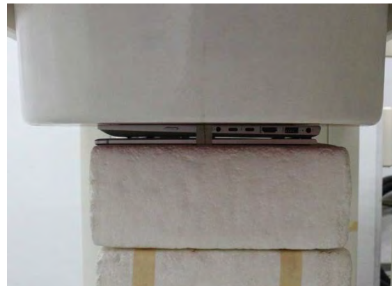
Fig.3 EUT Back side to flat phantom
