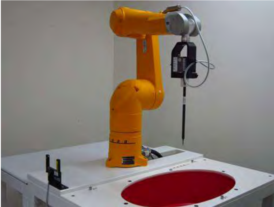
Fig.1 Photograph of the SAR measurement system
