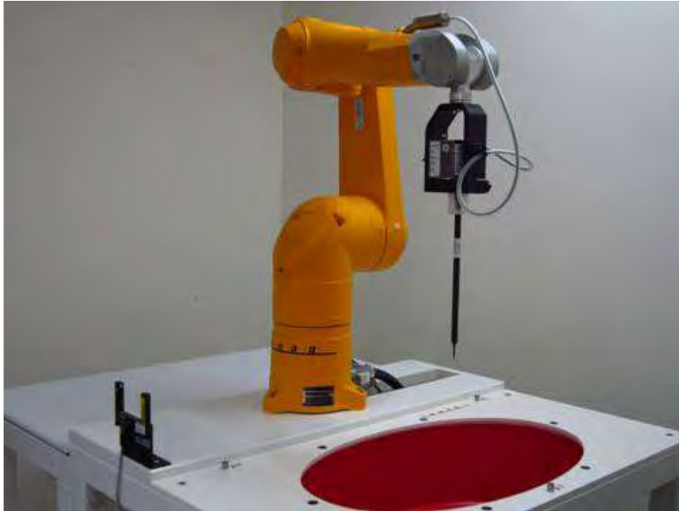
Fig.1 Photograph of the SAR measurement system
