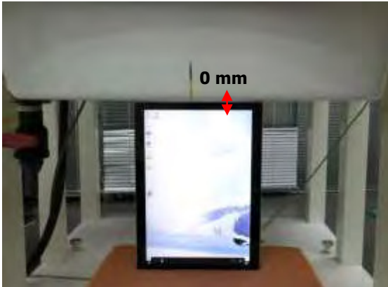
Fig.6 EUT Right side to flat phantom
