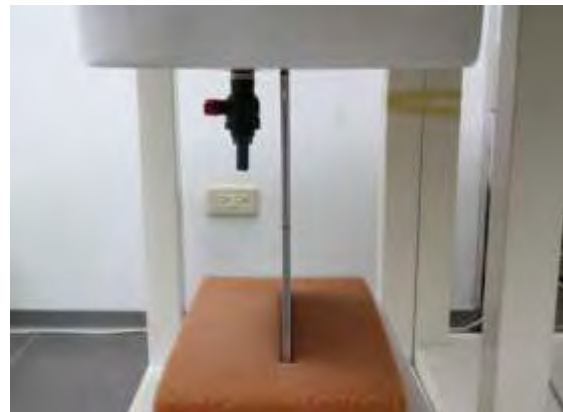
Fig.7 EUT Left side to flat phantom
