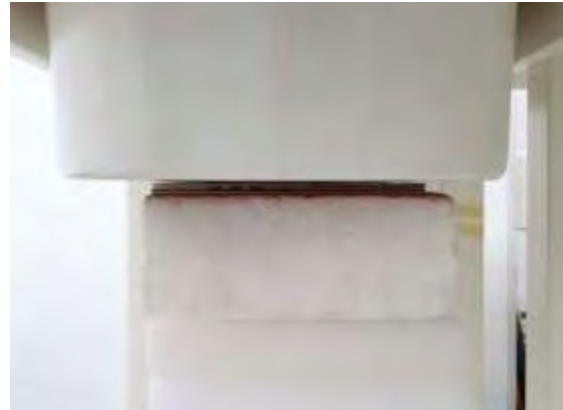
Fig.3 EUT Back side to flat phantom
