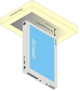
Fig-4.2 Illustration for Tablet Setup
