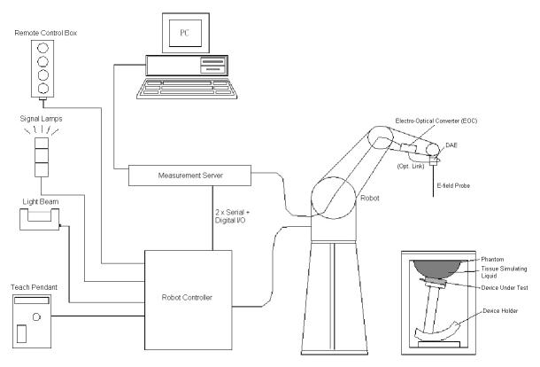
Fig-3.1 SPEAG DASY52 System Setup
