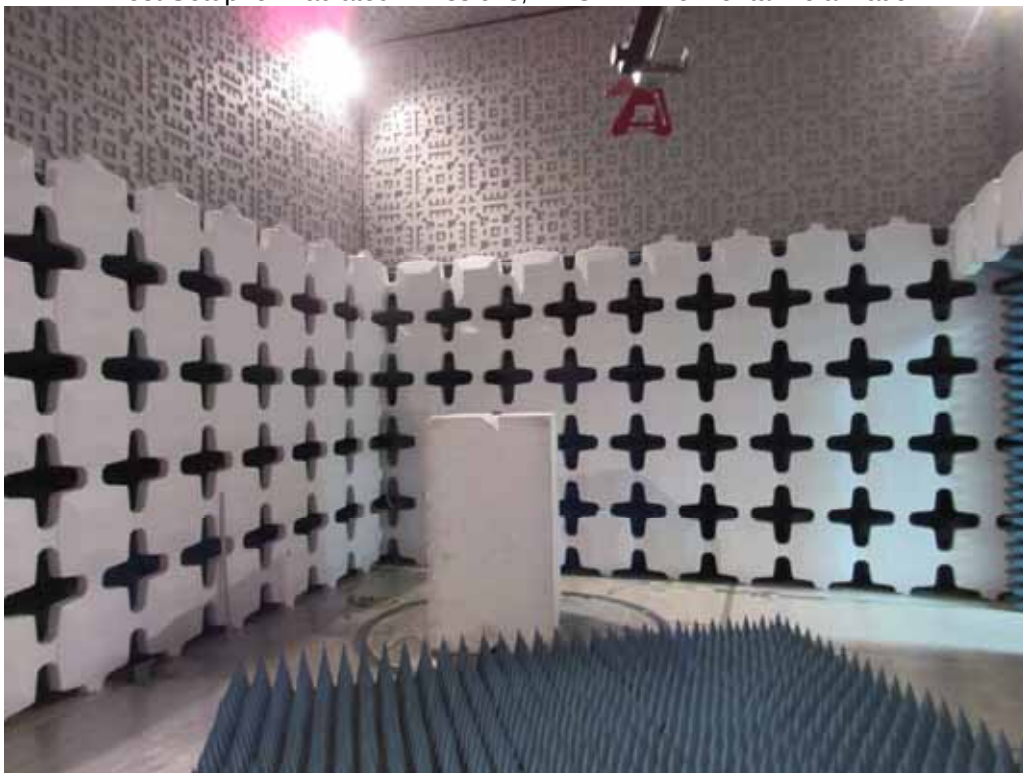
Test Setup for Radiated Emissions, 1-4GHz – Vertical Polarization
