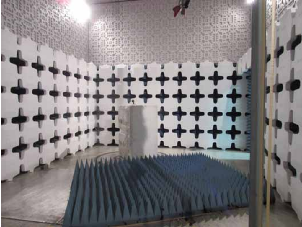
Test Setup for Radiated Emissions, 1 to 4.5GHz – Horizontal Polarization
