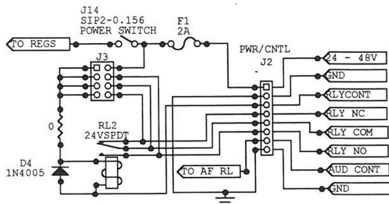
Relay RL2 is used for remote control of the transmitter input power supply. Header J3 allows the relay to be configured with jumpers so the relay coil can be energized by the main power input or any of the relay contacts. Diode D4 is the coil counter EMF diode.
