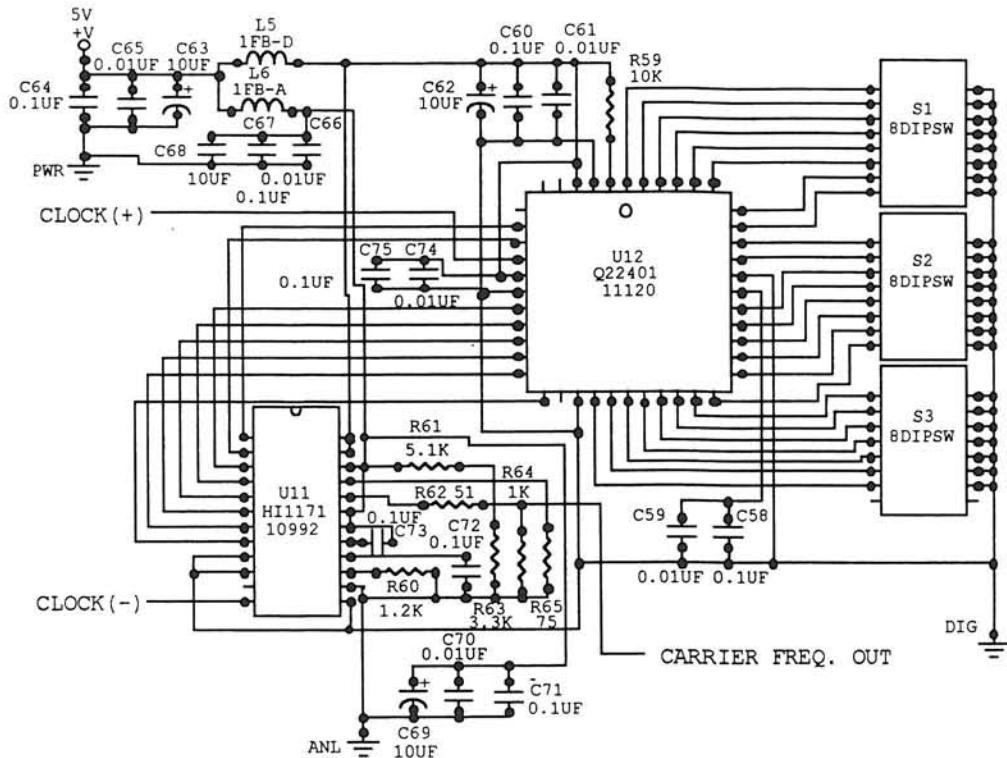
U12, a Q22401 direct digital synthesizer ASIC, along with U11, an eight bit D/A converter, generate the TR-6000 carrier frequency. DIP switches S1, S2 and S3 program the phase increment value for the desired carrier frequency. U12 generates the sine amplitude binary word output that is fed to U11's digital input. The sine amplitude value is converted into a sine waveform of the carrier frequency by U11.
