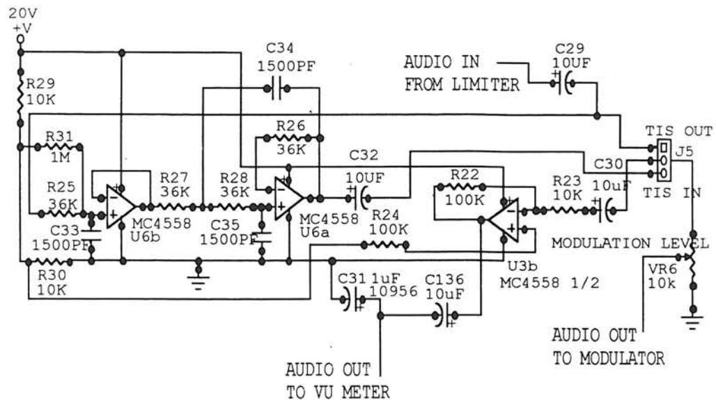
U6 is configured as a third order voltage-controlled voltage source low-pass filter. Resistor R25 and capacitor C33 form the first pole with a cutoff frequency of 2947Hz. U6b provides unity gain. The second pole, resistor R27 and capacitor C34, and the third pole, resistor R28 and capacitor C35, along with U6a form a unity gain second order low-pass filter with a cutoff frequency also of 2947Hz. U6b and U6a are cascaded to provide the -60dB per Decade roll-off required by the FCC regulations.
