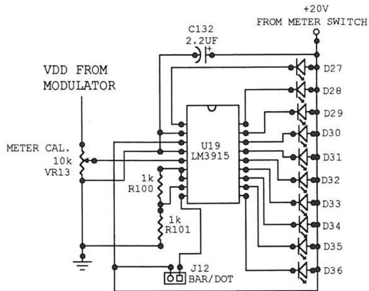
U19, an LM3915 logarithmic responding dot/bar display driver, senses analog voltage levels present on pin five (modulator VDD) and drives the ten LED's (D27 - D36) comprising the RF power output meter display. Meter calibration is accomplished by potentiometer VR13, with LED D34 representing 30 watts.
