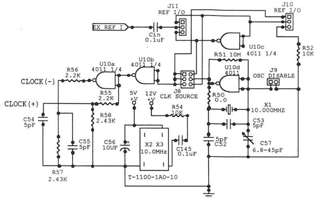
U10d and crystal X1 are configured as the standard inverter oscillator. The output is buffered and inverted by U10b producing the "Clock (+)" signal. Clock (+) is then inverted by U10a producing the "Clock (-)" signal. U10c is configured as an inverting buffer for X2 and X3 TCXO options and external GPS reference standards.
