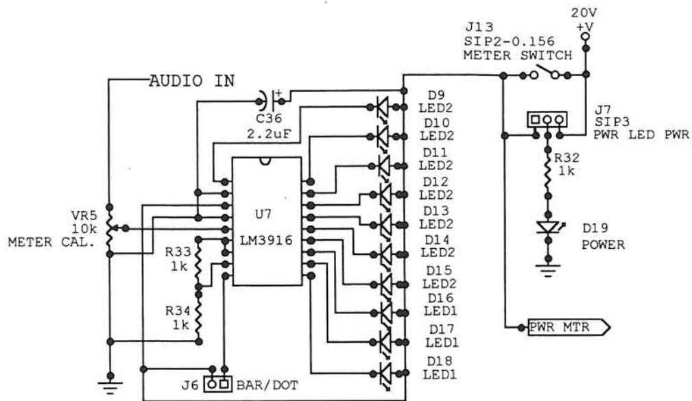
U7, an LM3916 VU responding dot/bar display driver, senses analog voltage levels present on pin five (modulation audio) and drives the ten LED's (D9 - D18) comprising the input audio VU meter display. Meter calibration is accomplished by potentiometer VR5, with LED D15 representing zero VU. LED D19 is the power present indicator.
