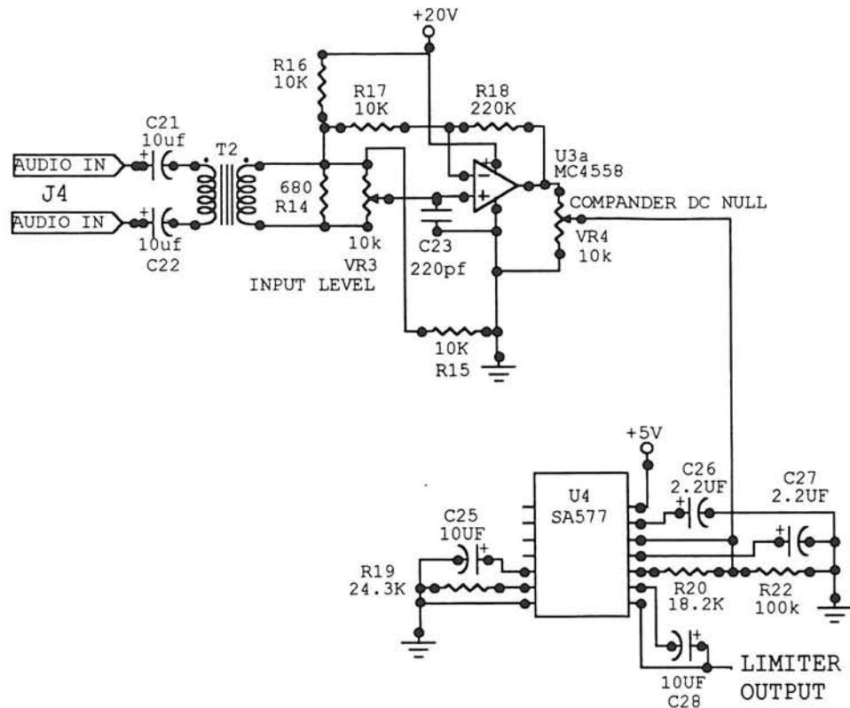
U3a is configured as a transformer isolated non-inverting amplifier with a variable gain of zero to twenty two. The output of U3a feeds the input of U4, an SA577 unity gain level compandor. The compressor side of U4 is configured as a feed-forward hard limiter with a fast attack time (22mS) and slow release time(88mS). The expander side of U4 is not used in this circuit.
