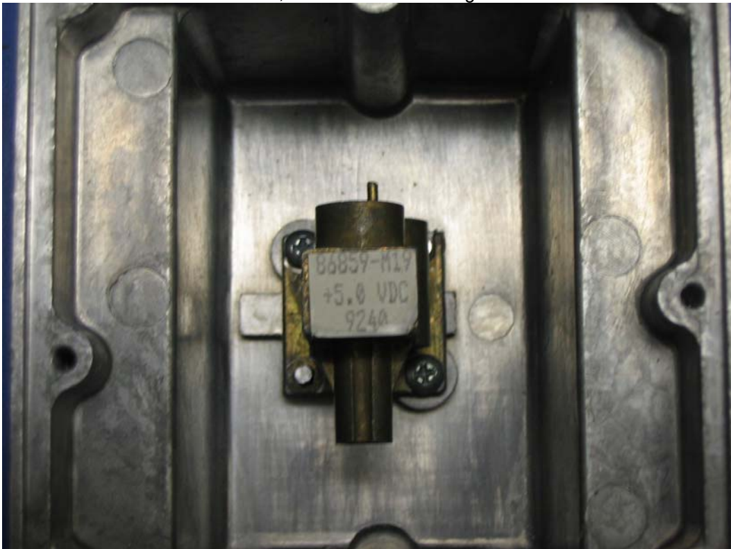
mn: 46783-1000, Transceiver in housing with out wires
