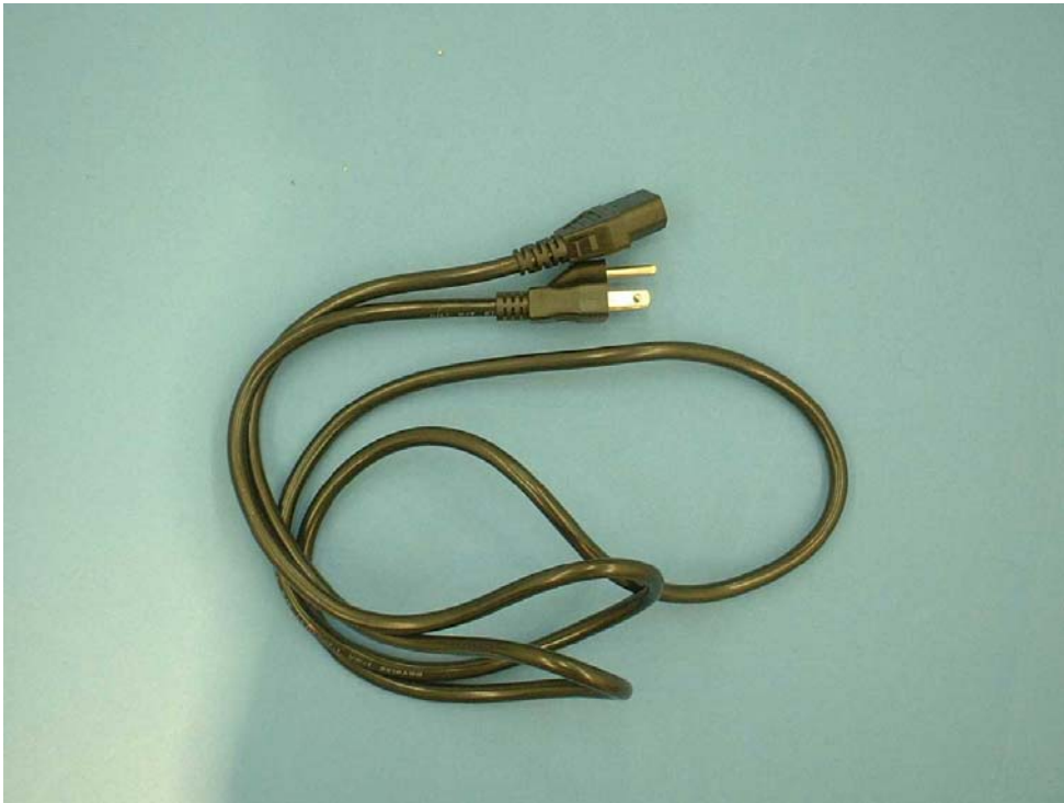
AC Main Cable
