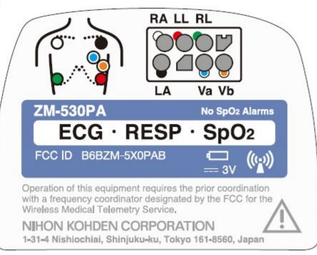
\*\*Since the test is conducted according to the requirements of IEC6061-1:1988/Amd1:1991/Amd2:1995 Section 6.1, the label will not peel off or the print will disappear during the product life.
