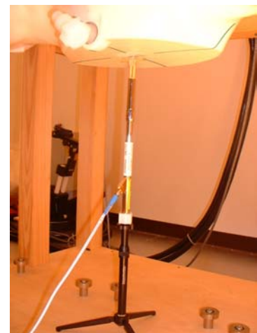
2450MHz System performance check setup
