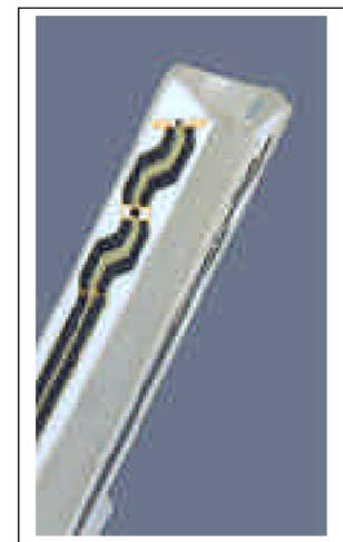
Inside view of ET3DV6 E-field Probe
