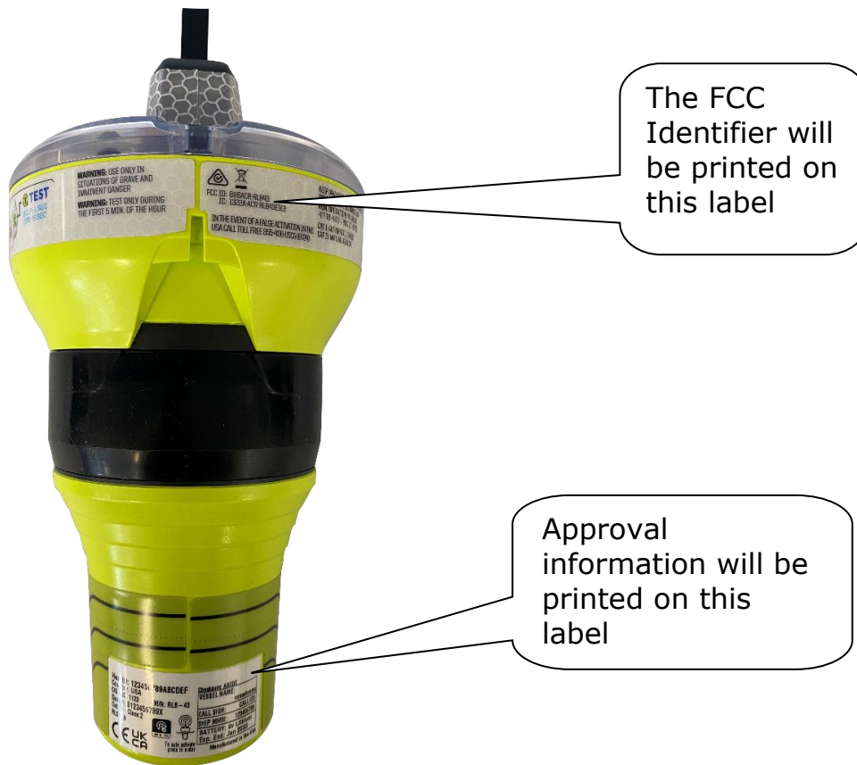
Figure 4: GlobalFix V6 – Rear View (Antenna Not Shown for Clarity)
