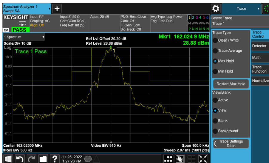
Figure 6 – 162.025 MHz - Transmitter Spectrum Mask
