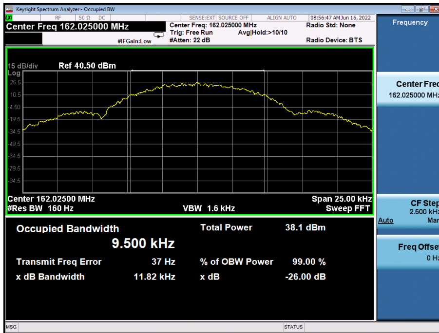
Figure 2 – 162.025 MHz Occupied Bandwidth
