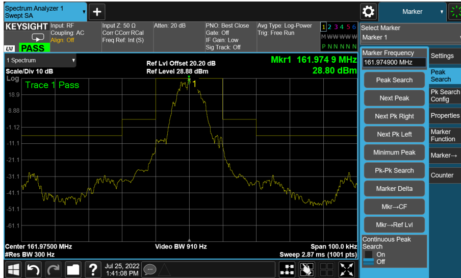
Figure 3 – 161.975 MHz - Transmitter Spectrum Mask
