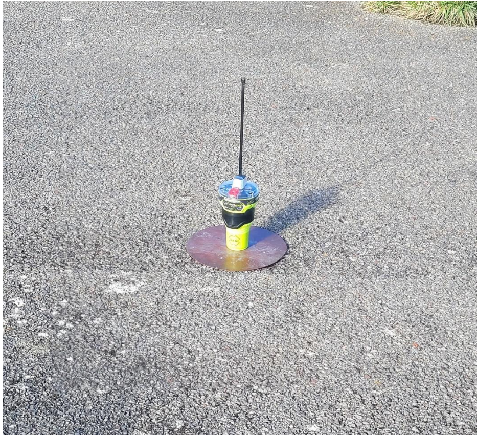
Satellite Qualitative Test – Configuration 7 GlobalFix V6
