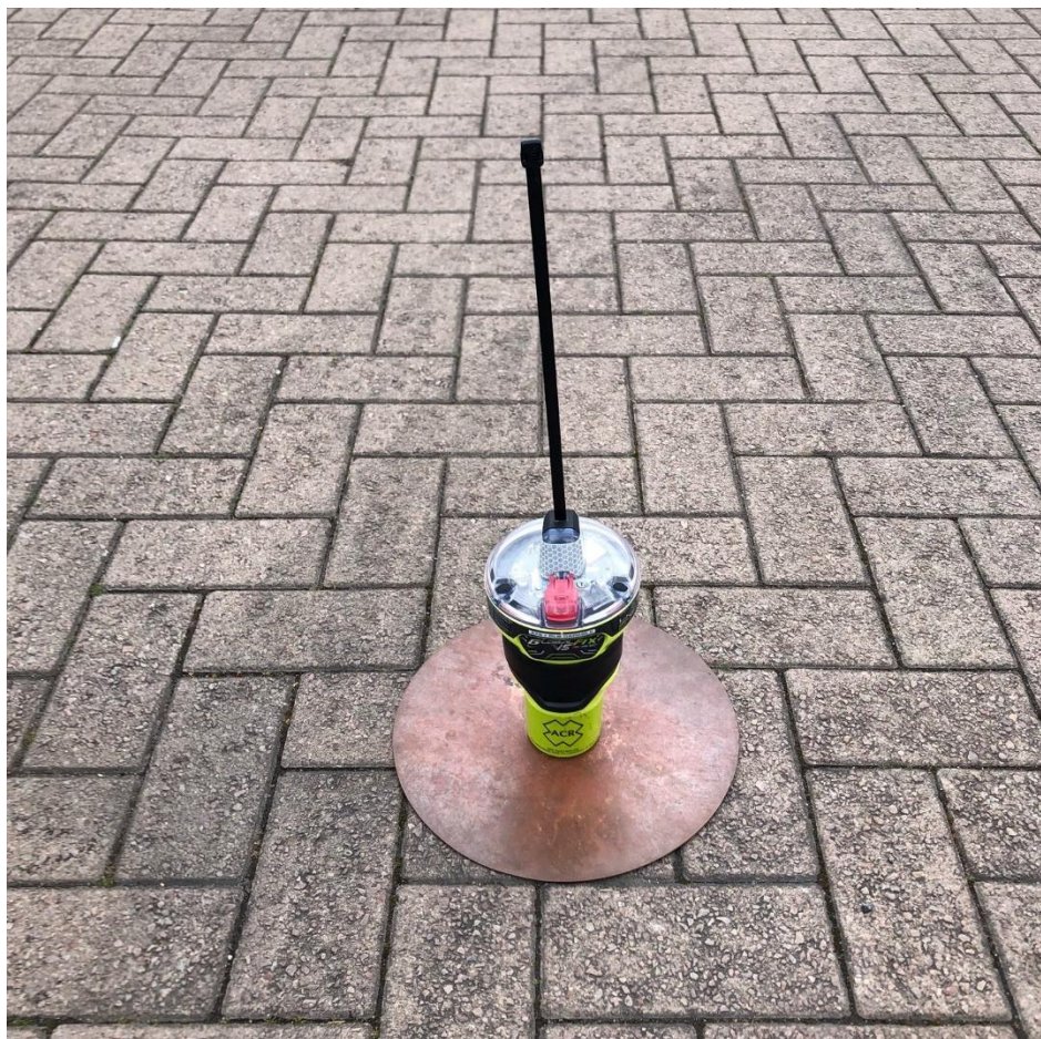
Position Acquisition Time and Position Accuracy Test – Configuration 7 – A.3.8.2.1 GlobalFix V6
