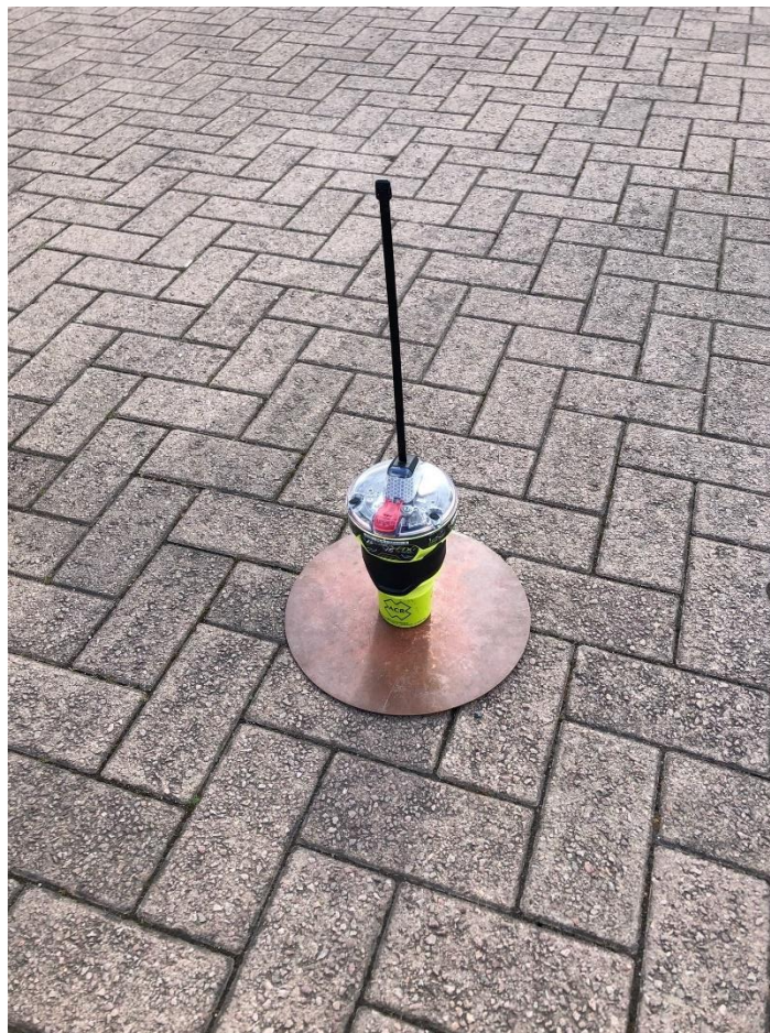
Position Acquisition Time and Position Accuracy Test – Configuration 7 – A.3.8.2.1 GlobalFix V6 Class 3
