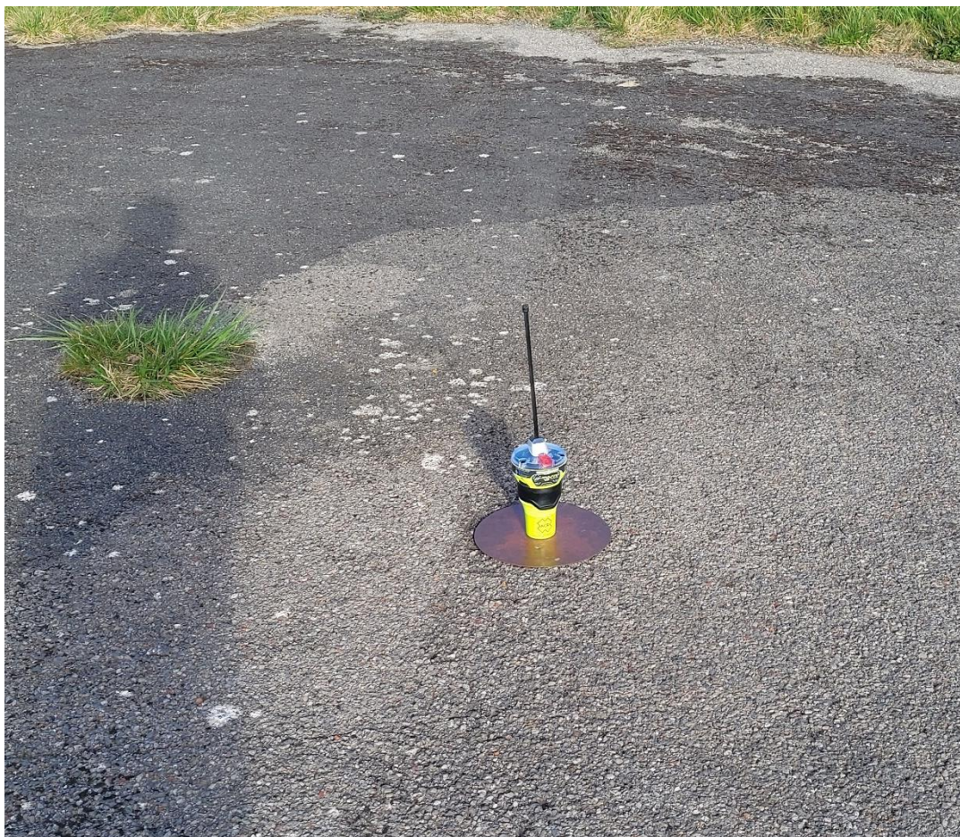
Position Acquisition Time and Position Accuracy Test – Configuration 7 – A.3.8.2.2 GlobalFix V6
