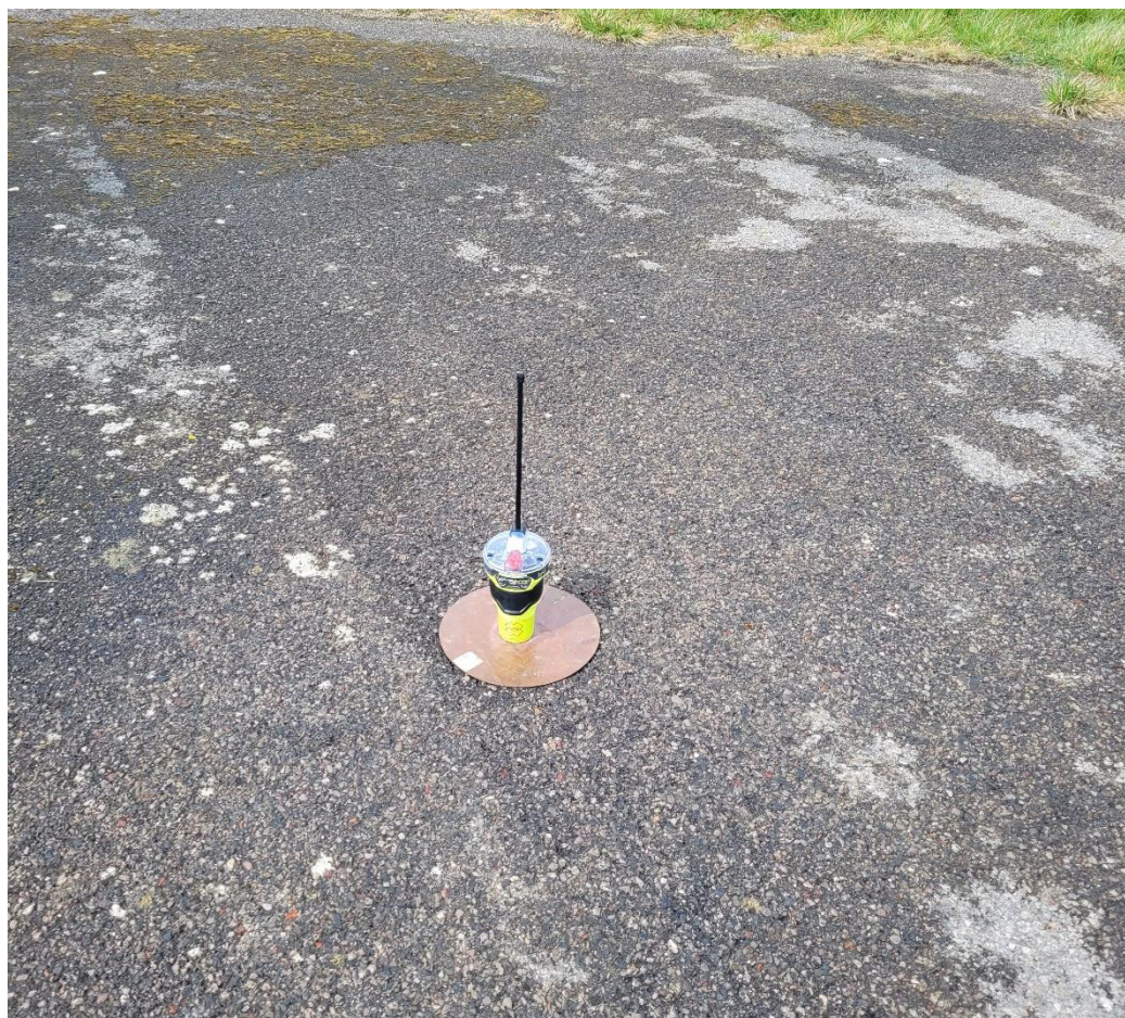
Position Acquisition Time and Position Accuracy Test – Configuration 7 – A.3.8.2.2 GlobalFix V6 Class 3
