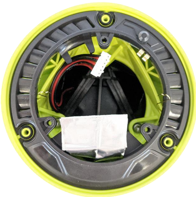
Figure 2: GlobalFix V5 – Top view, PCB removed showing battery carrier in-situ.
