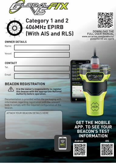
1,912grams (4.25lbs Portable Class 2 -20C to +55C Class 2 -30C to +70C 10m depth for 1 hou 4m maximum
