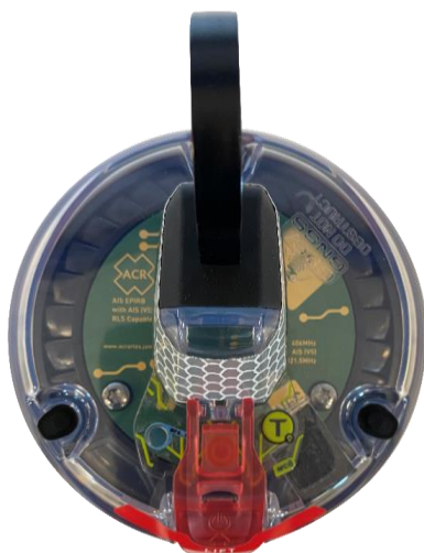
Figure 5: GlobalFix V5 - Top View Including Fixed Antenna in Stowed Configuration
