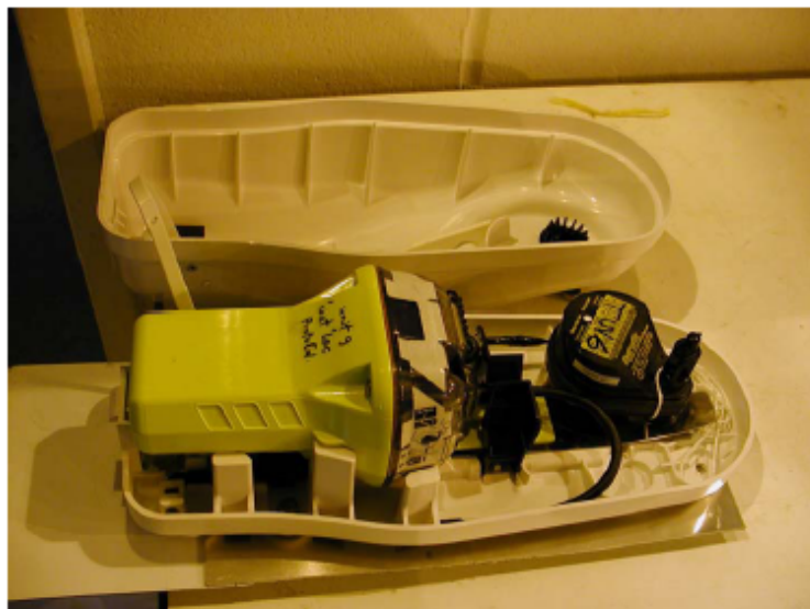
Figure 1: EPIRB with release mechanism primed
