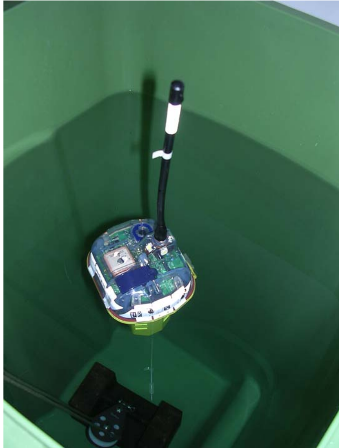
EUT Immersed In Fresh Water
