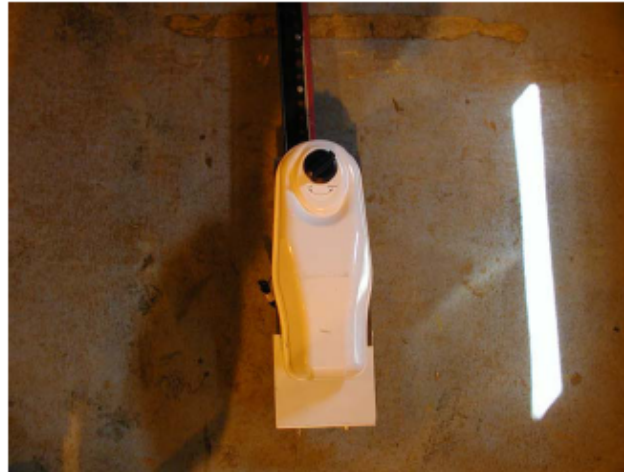
Figure 2: EPIRB mounted on the plunge pole ready for testing, Vertical Normal attitude.
