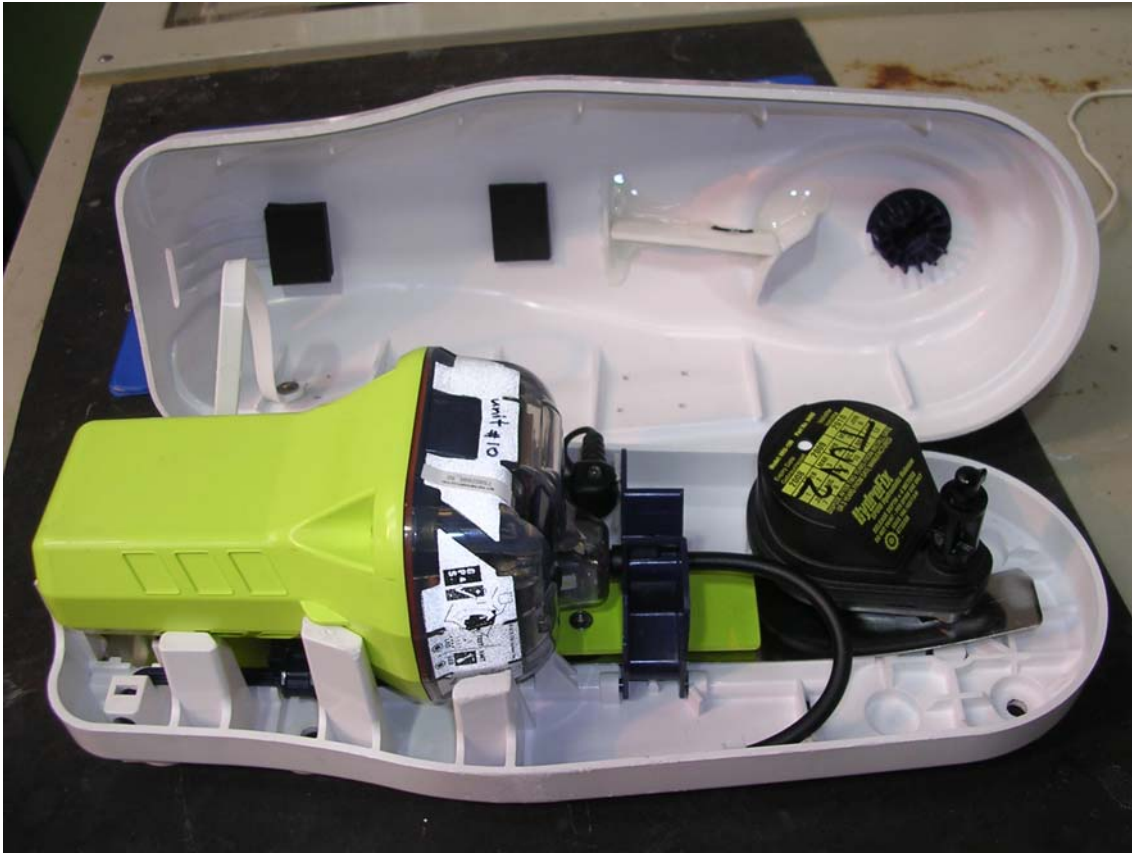
View of EUT: Unit #10 in release mechanism
