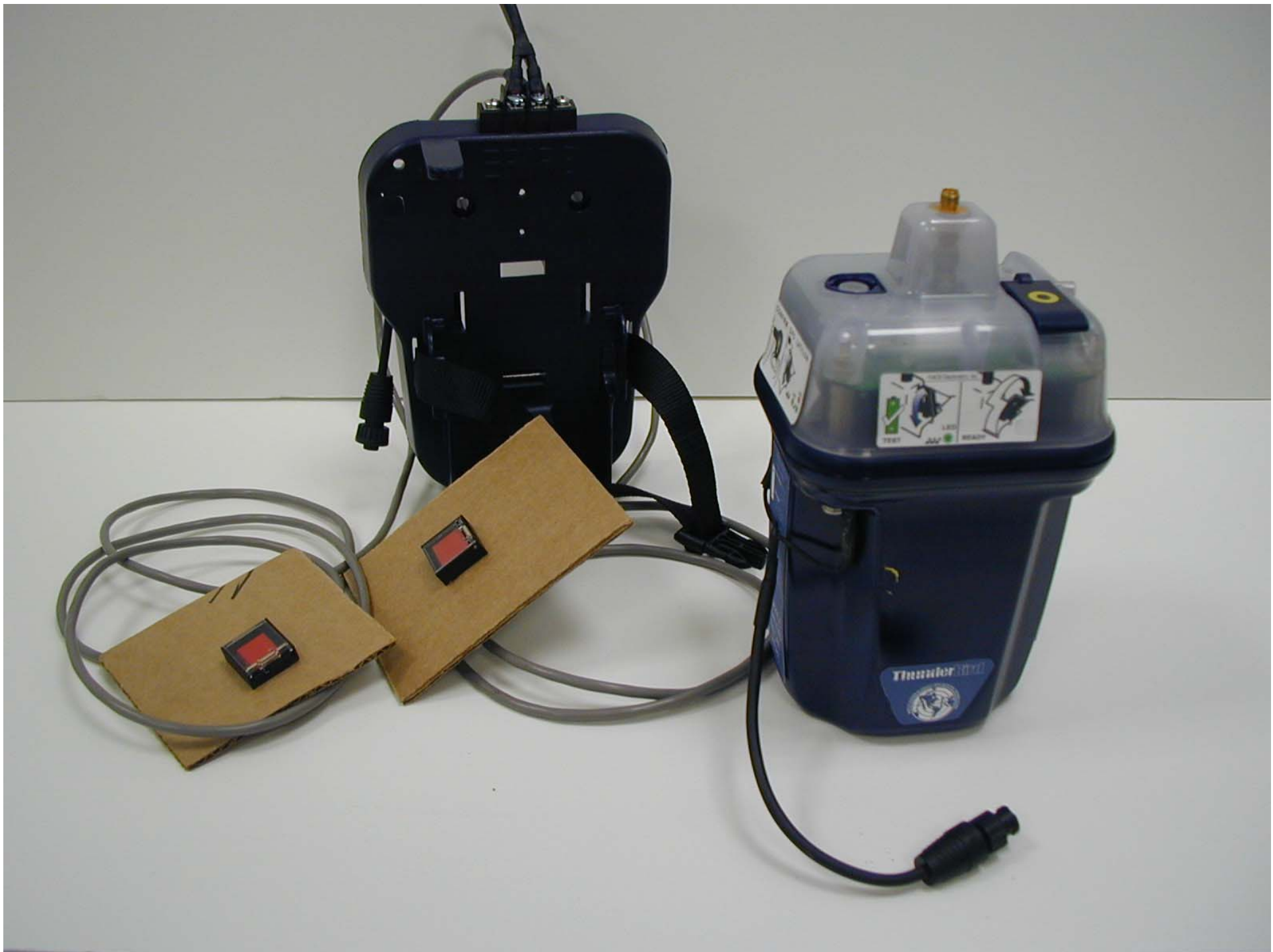
RLB-33S System: Beacon Removed
