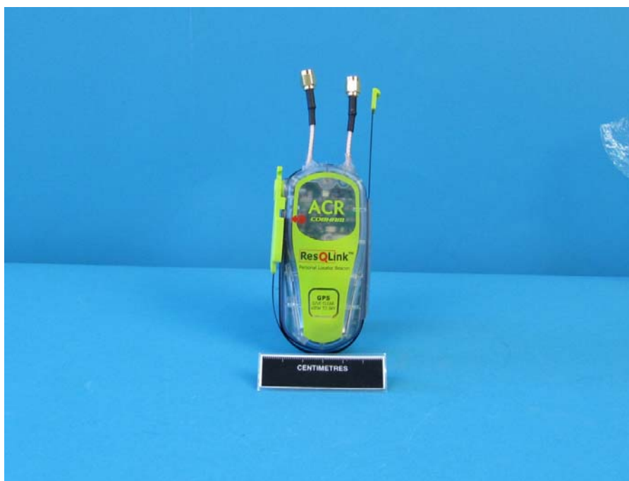
Test sample with 50Ω Antenna connectors
