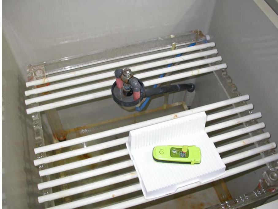
Photograph of EUT in the Salt Spray Chamber
