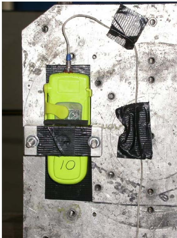
Photographs showing EUT mounted on Vibration machine
