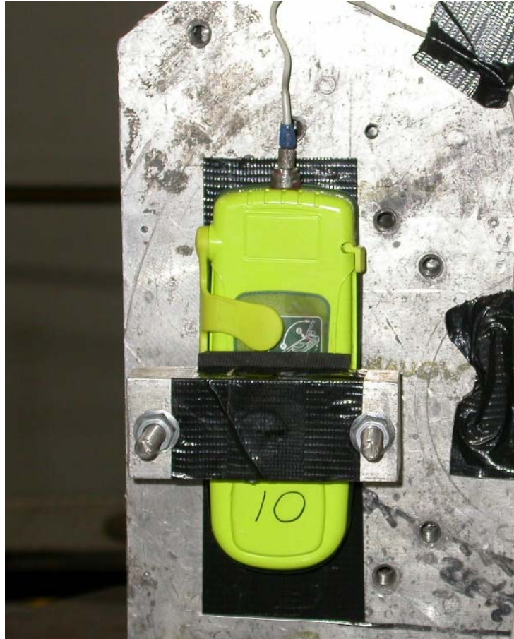
Photograph showing Ruggedness Test Set-up
