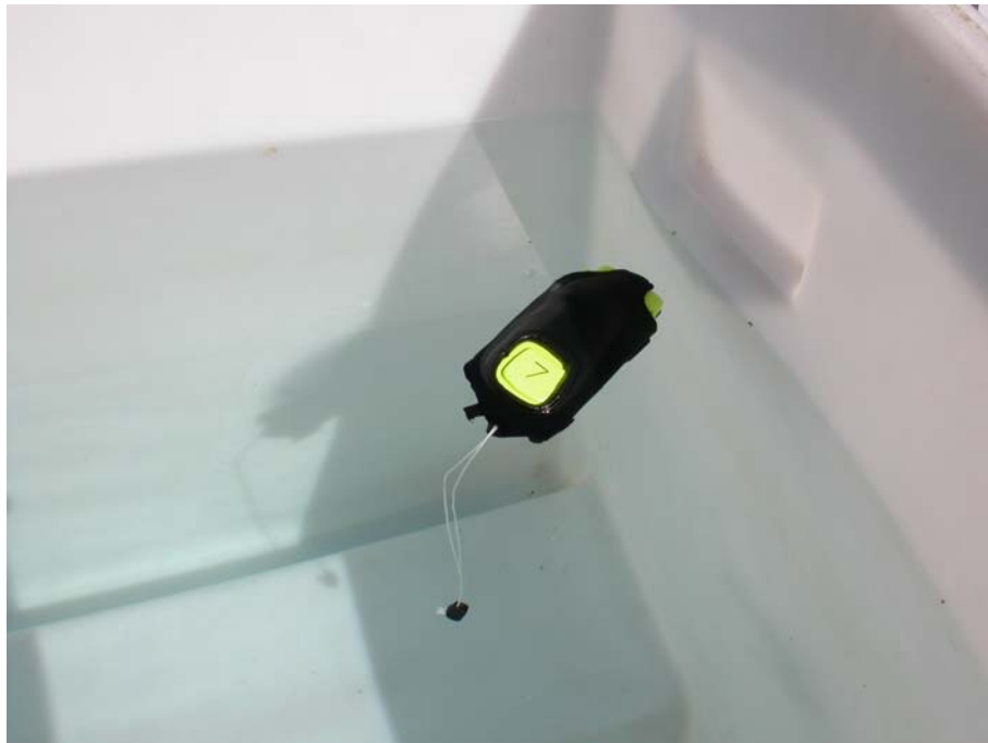
Photograph showing EUT (fitted with floatation pouch) floating in fresh water
