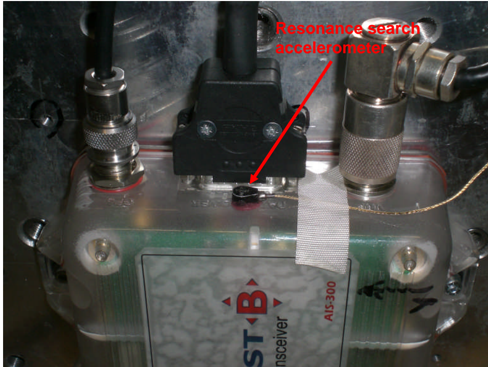
Picture 7: Resonance search accelerometer position X-Axis
