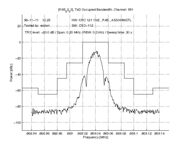
Referenced to the Rated Power Output at Lowest Level (- 20 dB) Modulated with 19.2 kbs PSEUDORANDOM DATA
