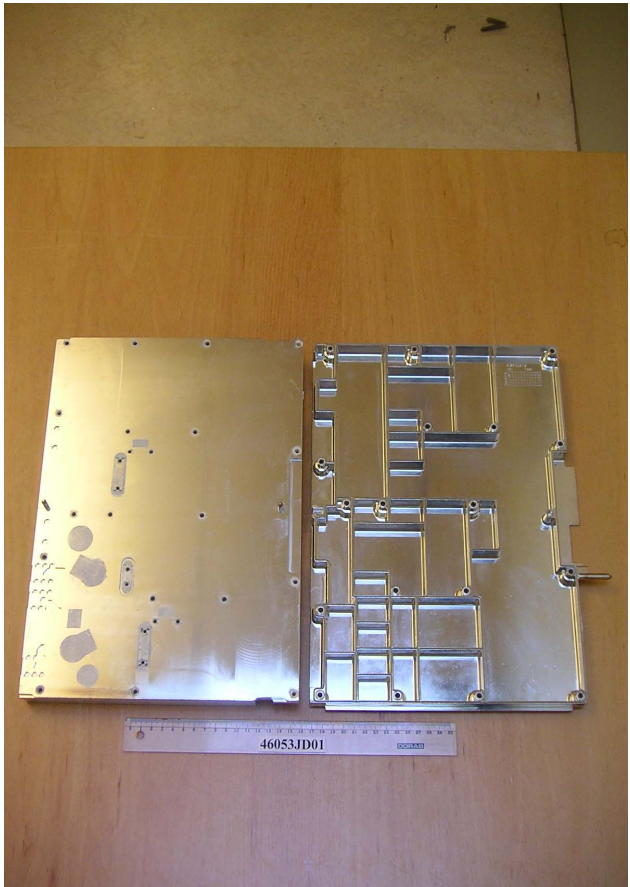
Internal view of removed heatsinks/casings
