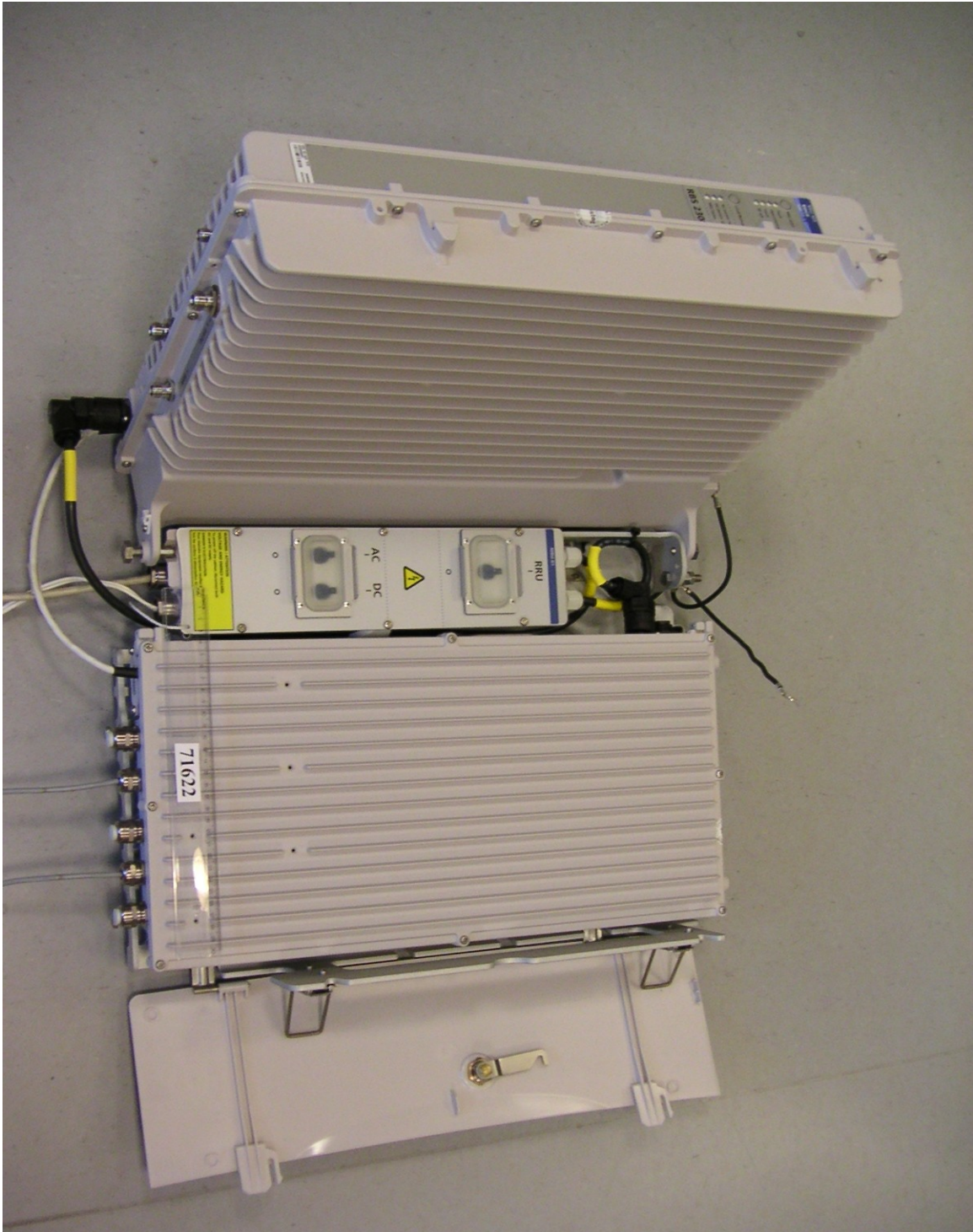
PHT/71622JD21/003 RBS2308 Cabinet with Mounting Base. Open View
