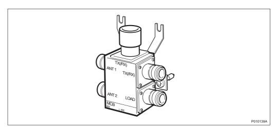
Figure 6 MCB antenna connection ports
