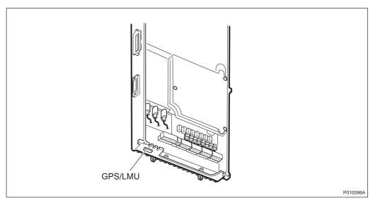
Figure 11 GPS/LMU connection port on IXU
