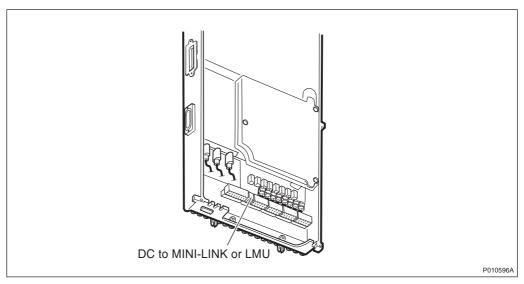
Figure 10 Location of MINI-LINK / LMU power supply in IXU
