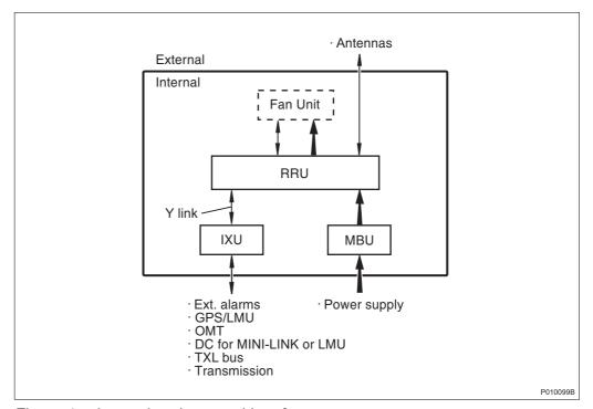
Figure 4 Internal and external interfaces
