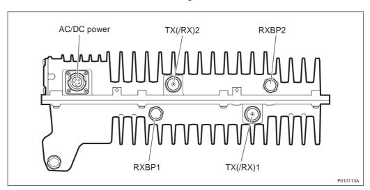
Figure 5 RRU antenna connections
