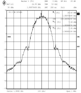
Testing for Ericsson AB. RBS2308 1900MHz. 45184JD06 Comment A: CH810. +29.5dBm. OBW 99% Occupied Bandwidth. 8PSK TXO. FCC 2.1049
