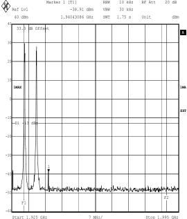
Testing for Ericsson AB. RBS2308 1900MHz. 45184JD06 Comment A: Ch 513&538. +33.5dBm. Conducted Spurious Emissions. 8PSK TX2/TX3. FCC Part 24.238
