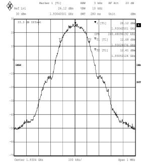
Testing for Ericsson AB. RBS2308 1900MHz. 45184JD06 Comment A: CH513. +33.5dBm. OBW 99% Occupied Bandwidth. GMSK TXO. FCC 2.1049
