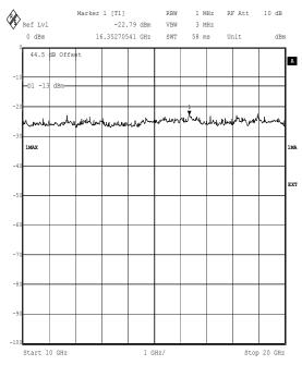
Testing for Ericsson AB. RBS2308 1900MHz. 45184JD06 Comment A: Ch 7846809 x33.5dBm. Conducted Spurious Emissions. 8PSK TXO/TX1. FCC Part 24.238
