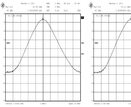
Testing for Ericsson AB. RBS2308 1900MHz. 45184JD06 Comment A: CH512. +30.2dBm. Output Power. 8PSK TX3. FCC Part 2.1046(a) Date: 19.SEP.2003 16:33:53 Date:
