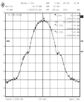
Testing for Ericsson AB. RBS2308 1900MHz. 45184JD06 Comment A: CH512. +29.5dBm. OBW 99% Occupied Bandwidth. GMSK TXO. FCC 2.1049
