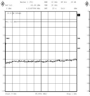
Testing for Ericsson AB. RBS2308 1900MHz. 45184JD06 Comment A: Ch 513&538. +33.5dBm. Conducted Spurious Emissions. GMSK TX0/TX1. FCC Part 24.238
