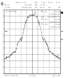
Testing for Ericsson AB. RBS2308 1900MHz. 45184JD06 Comment A: CH512. +33.5dBm. OBW 99% Occupied Bandwidth. 8PSK TXO. FCC 2.1049
