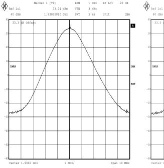
Testing for Ericsson AB. RBS2308 1900MHz. 45184JD06 Comment A: CH512. +33.5dBm. Output Power. GMSK TX2. FCC Part 2.1046(a) Date: 19.SEP.2003 15:48:27
