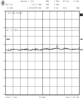
Testing for Ericsson AB. RBS2308 1900MHz. 45184JD06 Comment A: Ch 784&809. +33.5dBm. Conducted Spurious Emissions. 8PSK TX2/TX3. FCC Part 24.238
