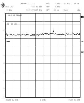
Testing for Ericsson AB. RBS2308 1900MHz. 45184JD06 Comment A: Ch 5134538 + 33.5dBm. Conducted Spurious Emissions. 8PSK TX2/TX3. FCC Part 24.238
