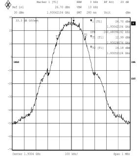
Testing for Ericsson AB. RBS2308 1900MHz. 45184JD06 Comment A: CH513. +33.5dBm. OBW 99% Occupied Bandwidth. GMSK TX2. FCC 2.1049
