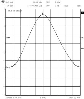
Testing for Ericsson AB. RBS2308 1900MHz. 45184JD06 Comment A: CH661. +30.2dBm. Output Power. 8PSK TX3. FCC Part 2.1046(a) 19.SEP.2003 16:35:48 Date:
