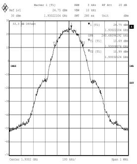
Testing for Ericsson AB. RBS2308 1900MHz. 45184JD06 Comment A: CH512. +31.5dBm. OBW 99% Occupied Bandwidth. GMSK TX2. FCC 2.1049
