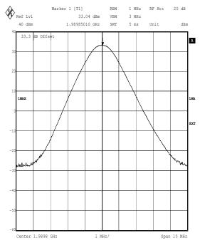
Testing for Ericsson AB. RBS2308 1900MHz. 45184JD06 Comment A: CH810. +30.2dBm. Output Power. 8PSK TX3. FCC Part 2.1046(a) Date: 19.SEP.2003 16:37:15
