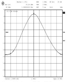
Testing for Ericsson AB. RBS2308 1900MHz. 45184JD06 Comment A: CH810. +33.5dBm. Output Power. GMSK TXO. FCC Part 2.1046(a) Date: 19.SEP.2003 15:30:10
