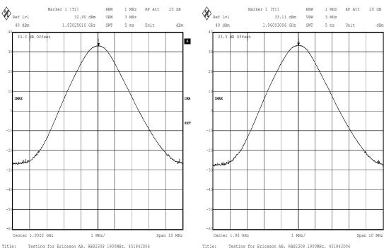
Testing for Ericsson AB. RBS2308 1900MHz. 45184JD06 Comment A: CH512. +33.5dBm. Output Power. GMSK TXO. FCC Part 2.1046(a) Date: 19.SEP.2003 15:24:58 Date:
