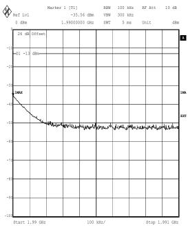
Testing for Ericsson AB. RBS2308 1900MHz. 45184JD06 Comment A: Ch 7846809 x33.5dBm. Conducted Spurious Emissions. 8PSK TX2/TX3. FCC Part 24.238
