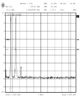
Testing for Ericsson AB. RBS2308 1900MHz. 45184JD06 Comment A: Ch 513&538. +33.5dBm. Conducted Spurious Emissions. GMSK TXO/TX1. FCC Part 24.238
