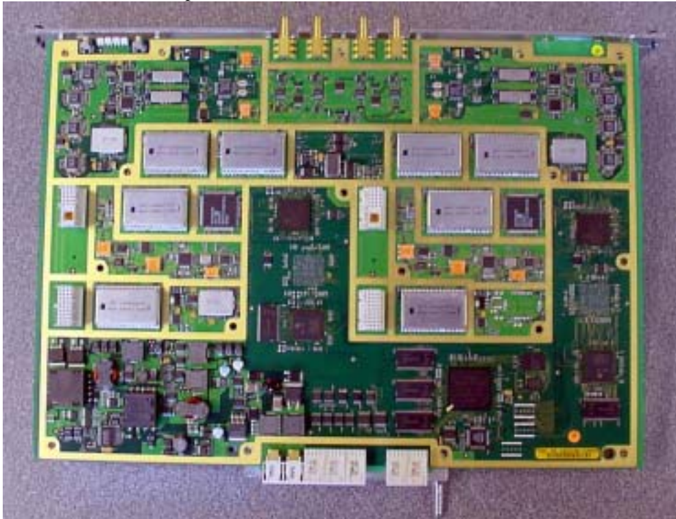
Main board- PCB rear side
