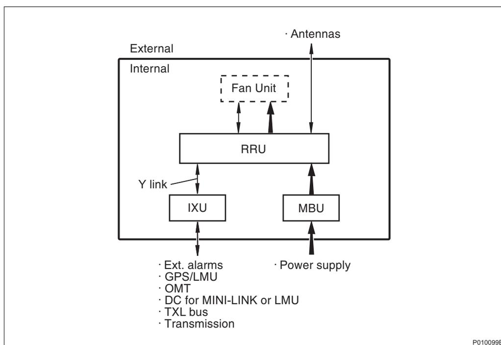
Figure 4 Internal and external interfaces
