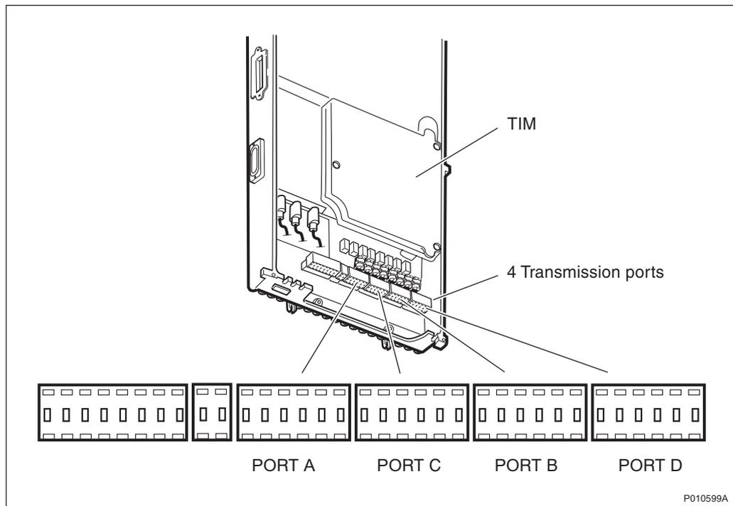
Figure 8 Location of T1 transmission ports in IXU
