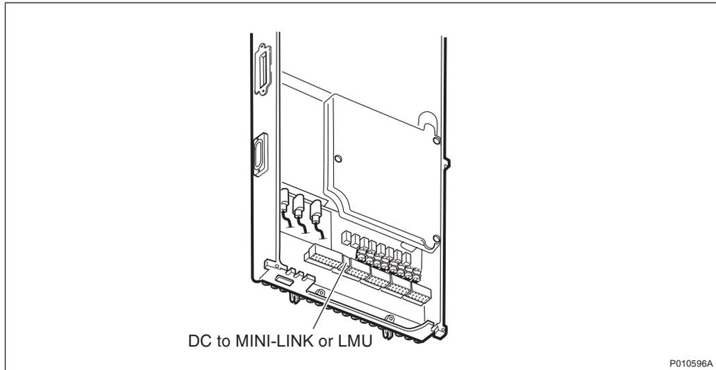
Figure 10 Location of MINI-LINK / LMU power supply in IXU
