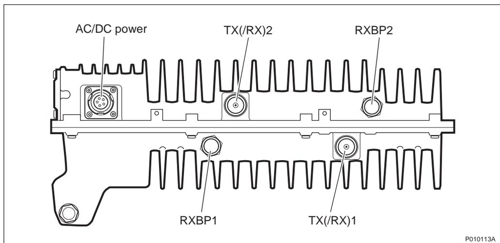
Figure 5 RRU antenna connections
