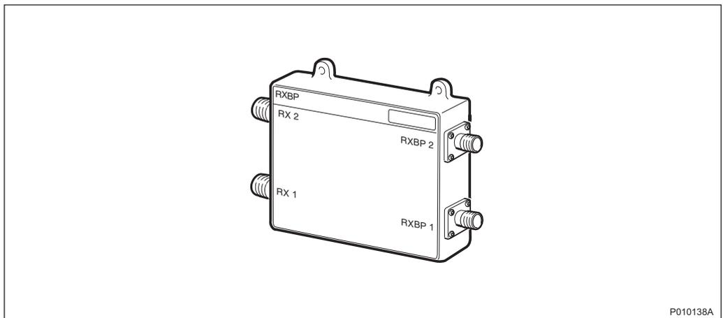
Figure 7 RXBP antenna connection ports
