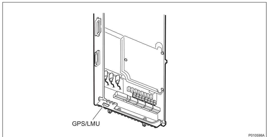
Figure 11 GPS/LMU connection port on IXU
