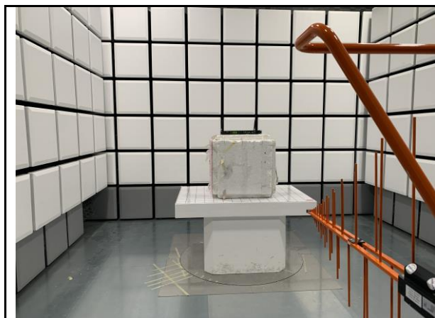
Radiated Emission Test below 30MHz Front View
