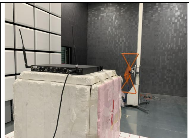
Radiated Emission Test below 30MHz Rear View
