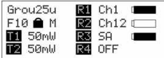
FIGURE 53. Status Screen with Lockout Active
