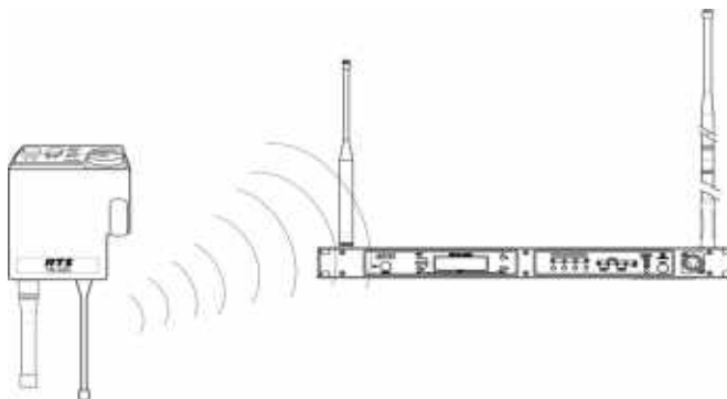
FIGURE 12. Vertically Polarized Antennas
