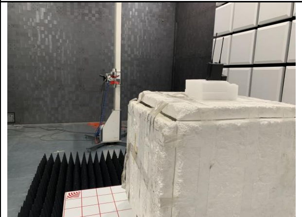
Radiated Emission Test below 1GHz Rear View
