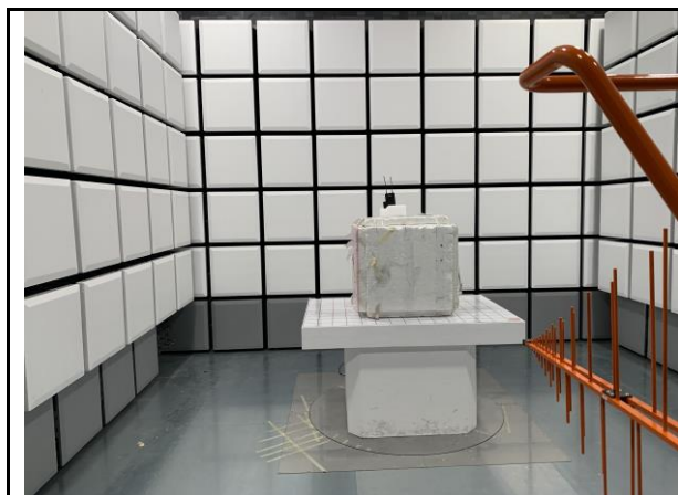
Radiated Emission Test below 30MHz Front View
