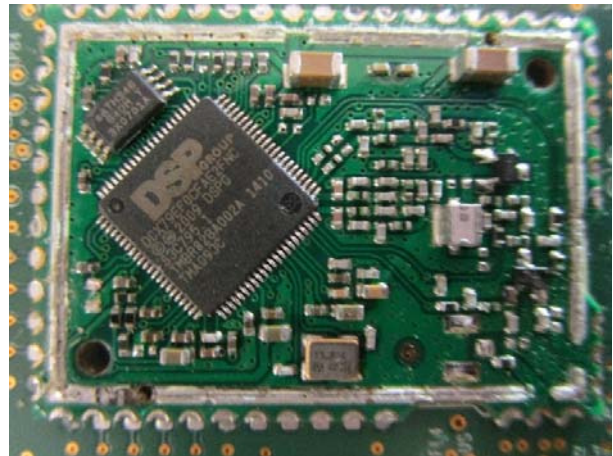
RF Module Cover Off View
