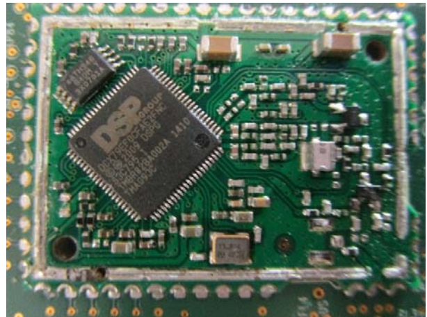
RF Module Cover Off View
