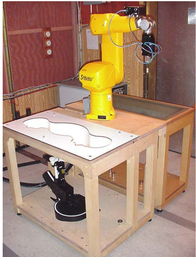
DASY4 SAR Measurement System with SAM phantom and device holder
