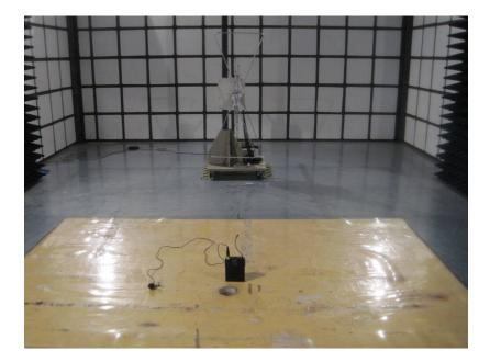
2.2 Radiation Emission Test View For 1GHz-10GHz
