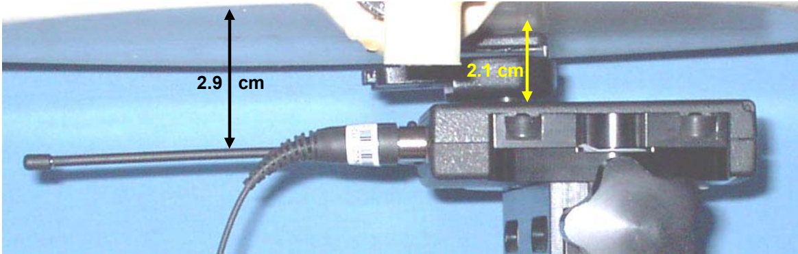
Low Channel Unit and Antenna (614 MHz)
