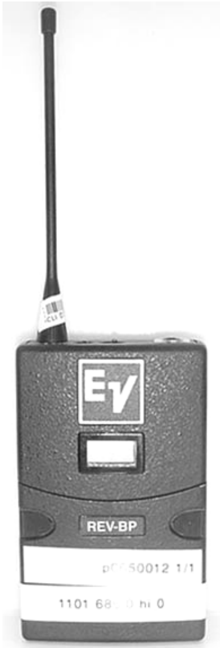
Front of DUT Mid Channel Unit (680 MHz)
