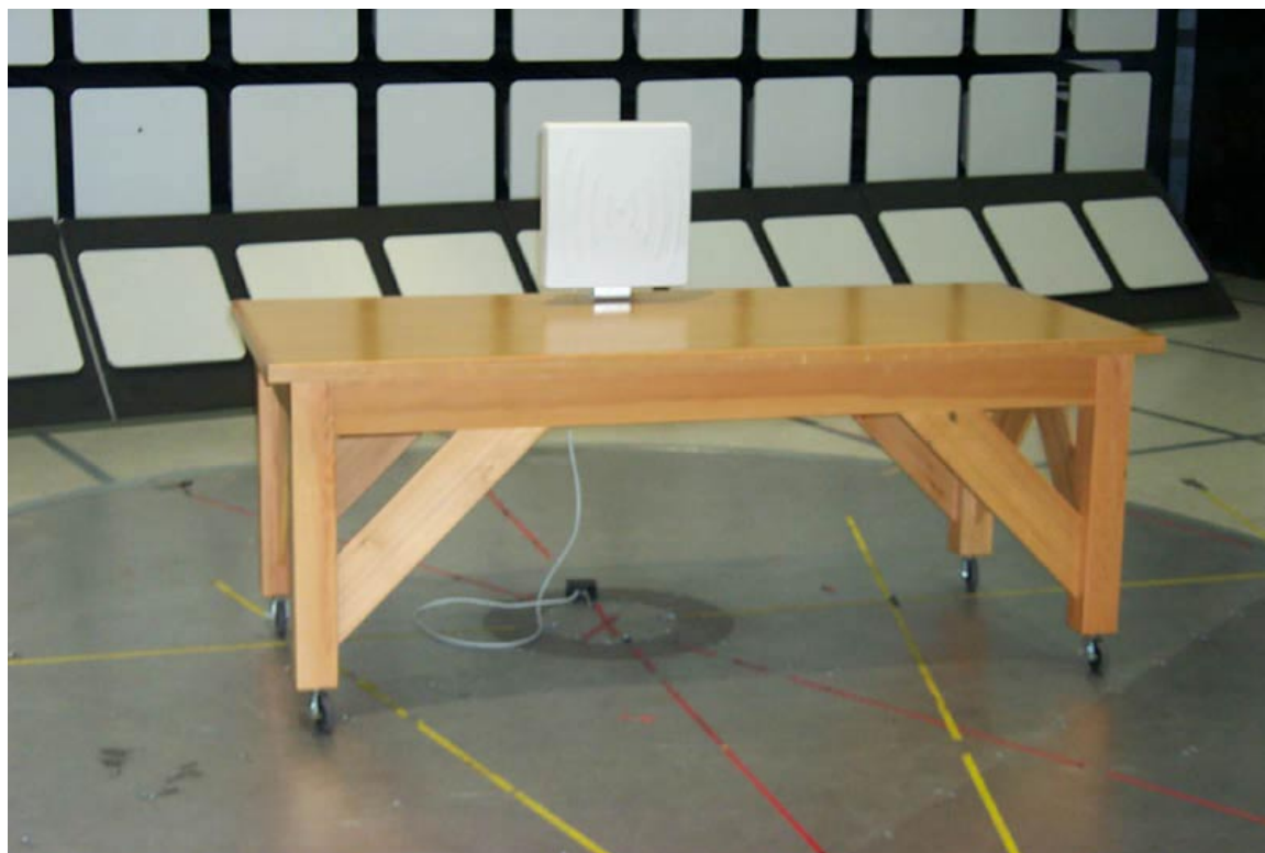
Figure 2 Radiated emissions test setup
