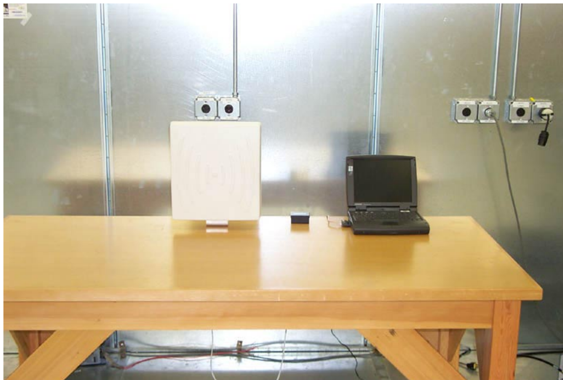
Figure 1 Conducted emissions test setup
