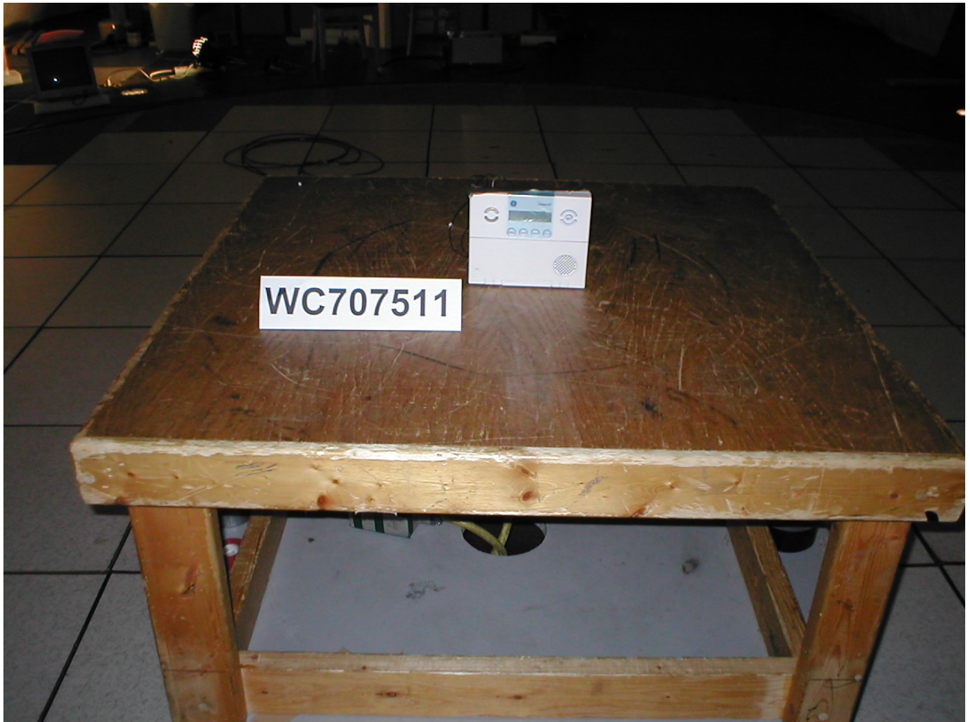
Test-setup photo(s): Radiated emissions
