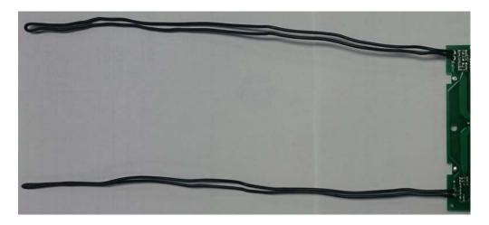
The antennas are made of stranded wire with black insulation with both ends soldered to PCB. The total length of each antenna is 22.4 cm. The design ensures that no antennas other than the one provided with the device shall be used with the intentional radiator.
